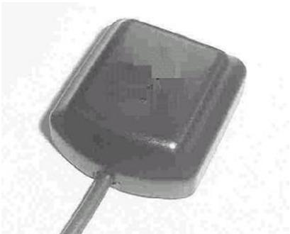
The window-mounting antenna is a convenient alternative for network time server applications if it is difficult to use a roof mounting antenna. Typically required accuracies in these applications are in the region of microseconds (or even milliseconds), and this performance can be delivered quite adequately from a reduced view of satellites down to just one.
